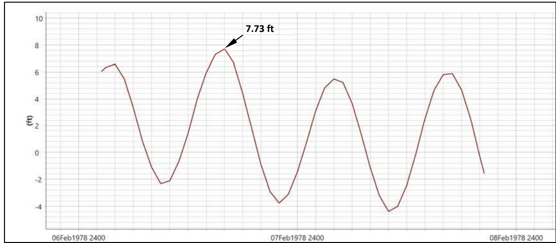
Figure 43 – Estimated 50-year tidal storm surge stage hydrograph used as the downstream boundary in the 50-year storm models without SLR
